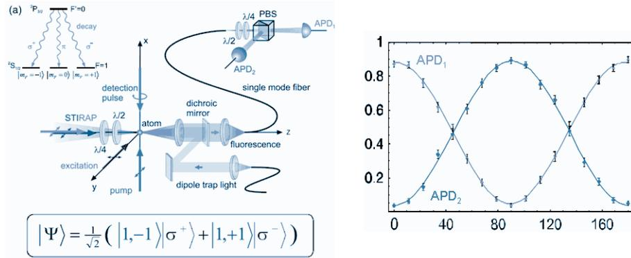
Figure 9: Atom photon entanglement, works even for bad cavities as the reconstruction may be conditioned on the detection of a photon. Can observe 87% fidelity [Volz, Weber et al.. PRL 96, 030404 (2006)].
