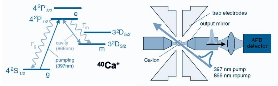
Figure 11: Level scheme and set-up for single photon source from a single ion trapped inside an optical cavity. [Keller, Lange, Hayasaka, Lange, Walther, NJP 6, 95 (2004); see also see focus issue for single photons on demand in New Journal of Physics 2004 (no subscription needed)].
