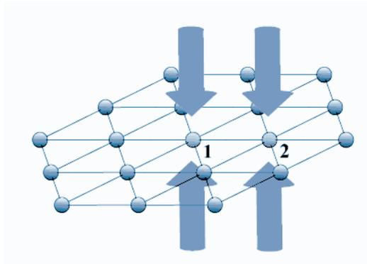
Figure 26: An 2-D ion crystal may be formed in a Penning trap and the oscillations of ion orthogonal to this plane may be used. Interactions may be induced for example via state-dependent dipole forces due to standing wave lasers. [Porras, Cirac, quant-ph/0601148]
