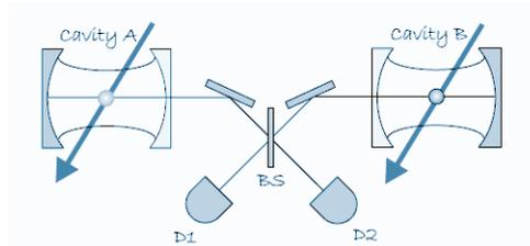
FIG. 1 (color online). We consider a setup in which individual ions are trapped inside two spatially separated optical cavities  $A$  and  $B$ . Photons can leak out of the cavities and are then mixed on a beam splitter  $BS$  and subsequently detected by photodetectors  $D_1$  and  $D_2$ .
