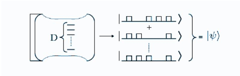
Figure 12: A trapped D-level atom is coupled to a cavity qubit, determined by the energy eigenstates  $|0\rangle$  and  $|1\rangle$ . After bipartite source-qubit operations, photonic time-bins are sequentially and coherently emitted at the cavity output, creating a desired entangled multi-qubit stream. [Schön, Hammerer, Wolf, Cirac, Solano, quant-ph/0612101]
