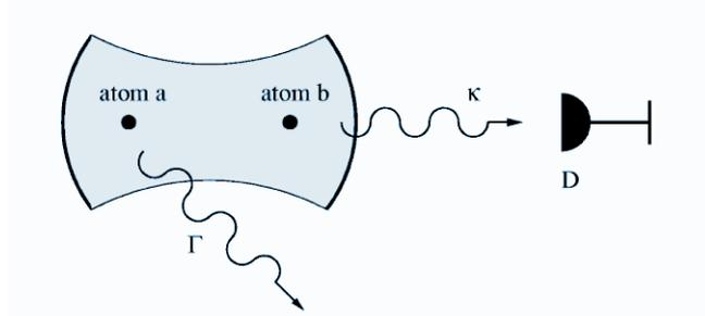
FIG. 1. Experimental setup. The system consists of two two-level atoms placed inside a leaky cavity. The decay rate  $\Gamma$  describes the spontaneous emission of the atoms, while the rate  $\kappa$  refers to photons leaking through the cavity mirrors. The latter can be monitored by the detector  $D$ .
