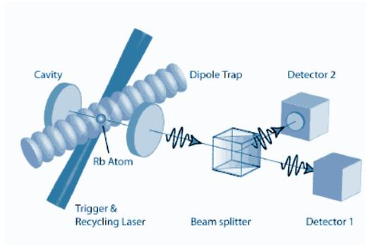
Figure 10: A single  $^{85}\text{Rb}$  atom is trapped in a high-finesse optical microcavity by means of a two-dimensional optical lattice. The atom-cavity system is excited by a sequence of laser pulses and single photons emitted from the system are detected by two avalanche photodiodes in Hanbury Brown & Twiss configuration. [Hijlkema, Weber, Specht, Webster, Kuhn, Rempe, quant-ph/0702034]
