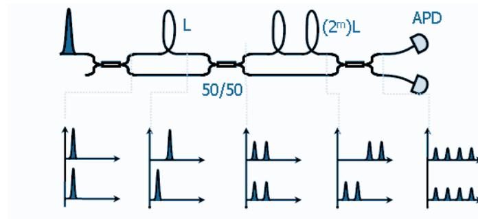
Figure 2: Fibre based beam-splitters with delay lines are used to split up wave packets which are then measured by standard yes/no avalanche photo-detectors.
